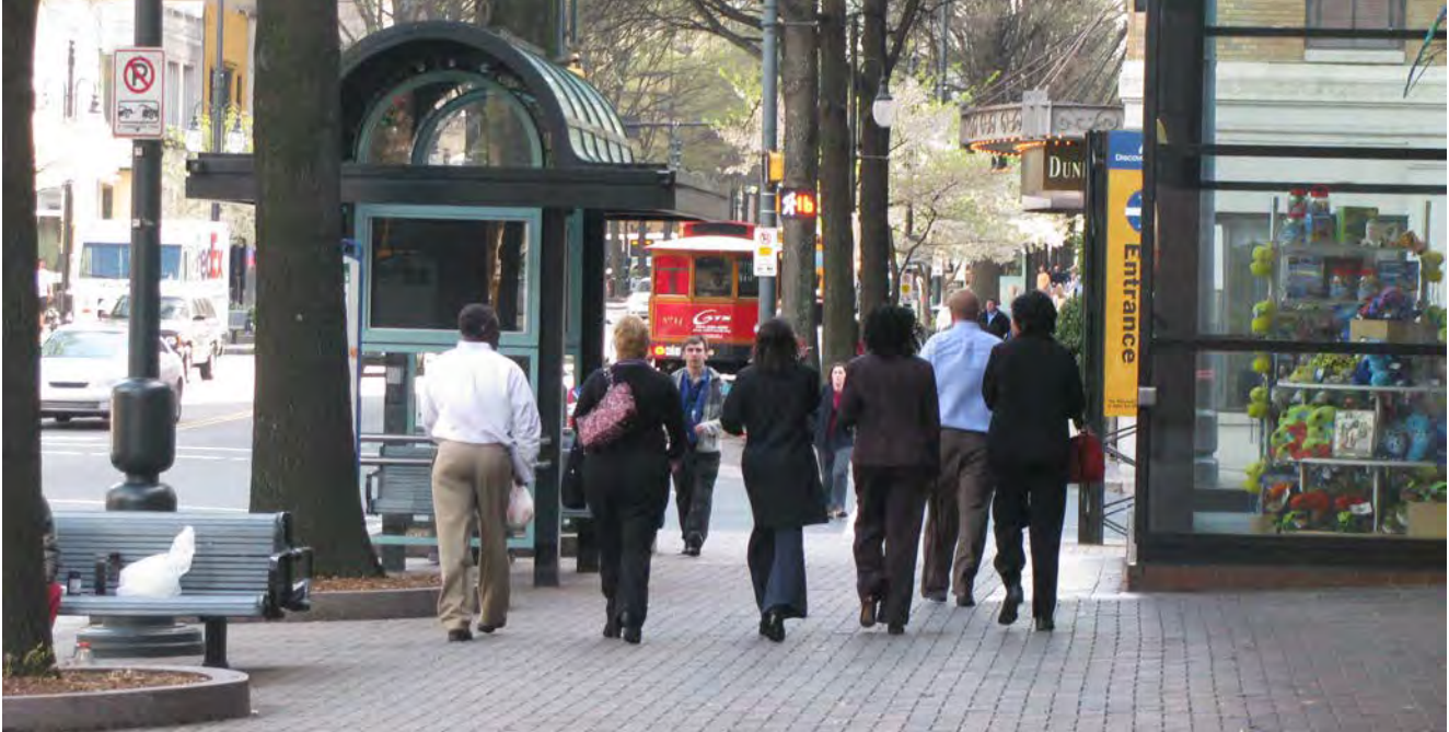
Sidewalk in Charlotte, NC, illustrating clear walkspace, plantings, and amenities. Courtesy of www.pedbikeimages.org / Dan Burden.
