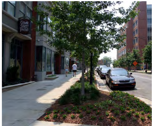
Planted buffers between pedestrians and cars not only improve the aesthetics of the street, but also its safety. Plants buffer walkers from traffic noise, and the flow of traffic, by designating a clear pedestrian corridor. Courtesy of Dan Burden, www.pedbikeimages.org .
